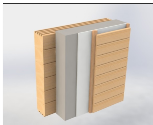
Image. Insulated solid wood wall
